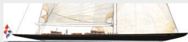
J Boat Lionheart : Delivery 2010 Designer Hoek Design Builder Claasen Jachtbouw LOA 43.4m LWL 26.51m Beam 6.55m Draft 4.8m
